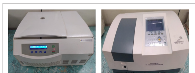
Figure 1) ) Centrifuge machine and UV-VIS spectrophotometer for biochemical analysis
